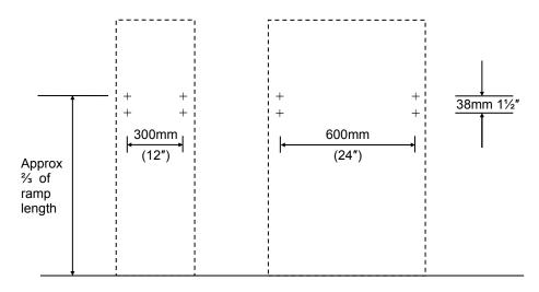
The crosses marked are location of the retainer clip screw holes.
